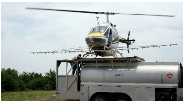
Figure 3. Helicopter equipped for aerial application.
