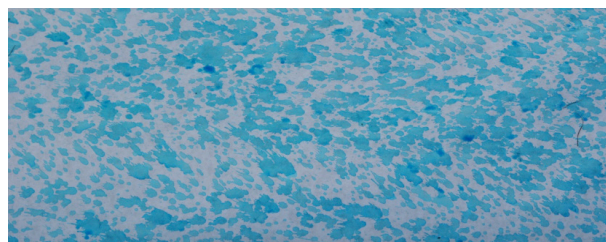
Figure 5. Boomless sprayer distribution pattern of a Boom Buster model 125 at 20 gallons per acre. Note the larger droplet size and uneven distribution.
